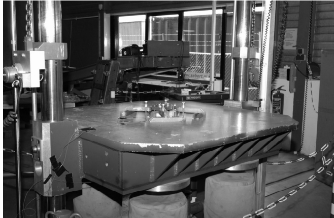
Figure 6.8 Beamsplitter shock testing on a drop table
