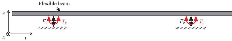
Figure 1.9: Flexible beam with torque production for vibration control (setup 2).
