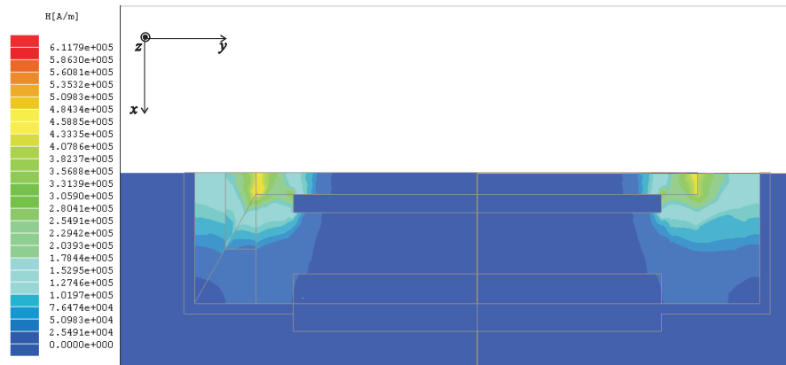
Figure 3.29: Modulus of the magnetic field intensity produced by the torque magnet in the xy -plane (FEM with the data-sheet magnets).
