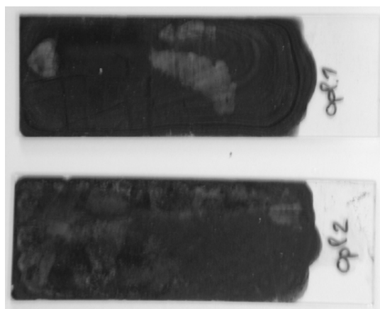
Figure 6.3 Photograph of filmcasted octadecanethiol stabilised nanoparticle / PMMA coatings
