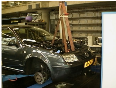
Figure 11.17: Engine compartment of the VW Bora test-car with built in ZI-CVT
