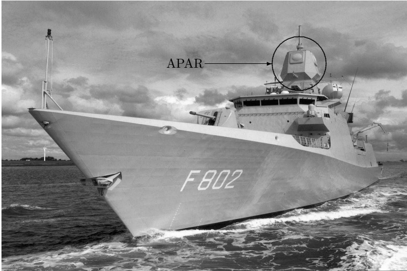
Figure 1.2: Complete operational APAR antenna on top of the latest LCF frigate of the Royal Dutch Navy.
