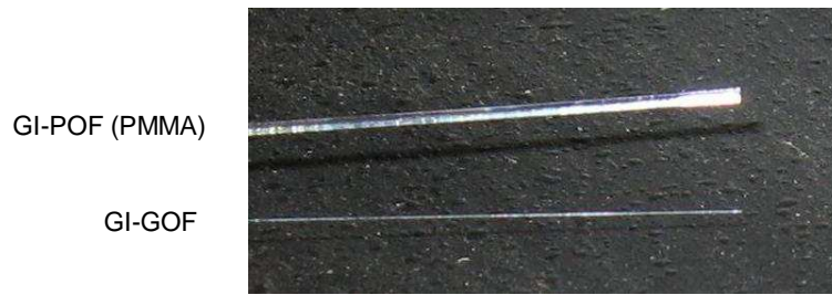
Figure 1.6: Photograph of two bare GI-MMFs; one GOF and one PMMA-POF.
