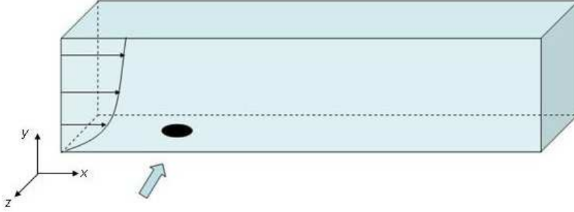
Figure 2.2: Sketch of the computational domain. Arrow indicates cooling jet.
