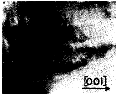
FIG. 2. A wide-beam-transmission topograph from a selenium single crystal with a 003 reflection. Dislocations of small-angle boundaries (dark in the figure) are visible at the point of the arrows. Magnification 20.
