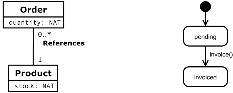
Figure 2: The UML class diagram of the trivial ordering system and the UML state diagram for the class Order .
