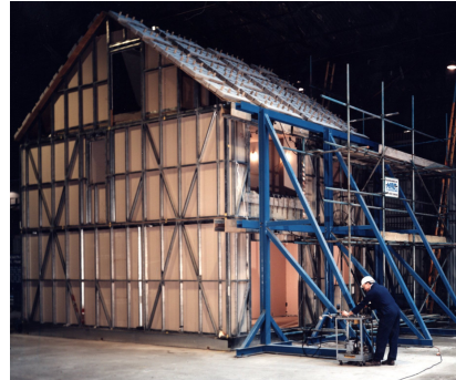
Figure 2. Testing of light steel frame
