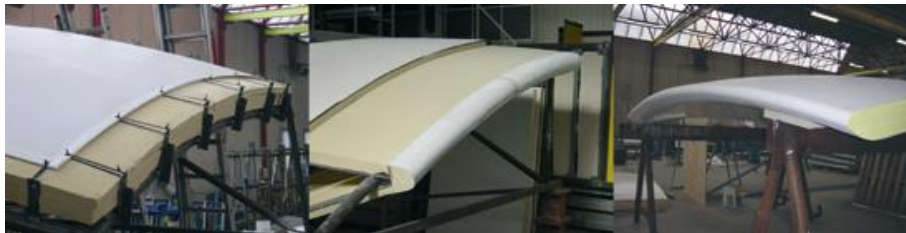
Figure 4. Three prototypes. Stressed membrane (left), GRP cladding to be locally produced (centre), prefab GRP sandwich (right)
