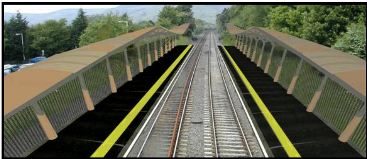
Figure 8: Wavy canopies achieved by using the ball-joint canopy-column connection
