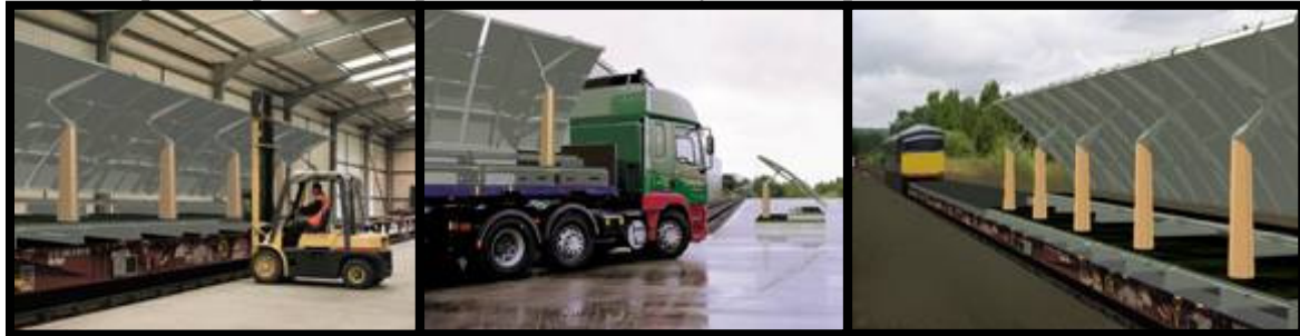
Figures 1,2,3. Adaptability to different access conditions: 2.4x2.4x2.7m module dimensions allow transportation on road and rail
