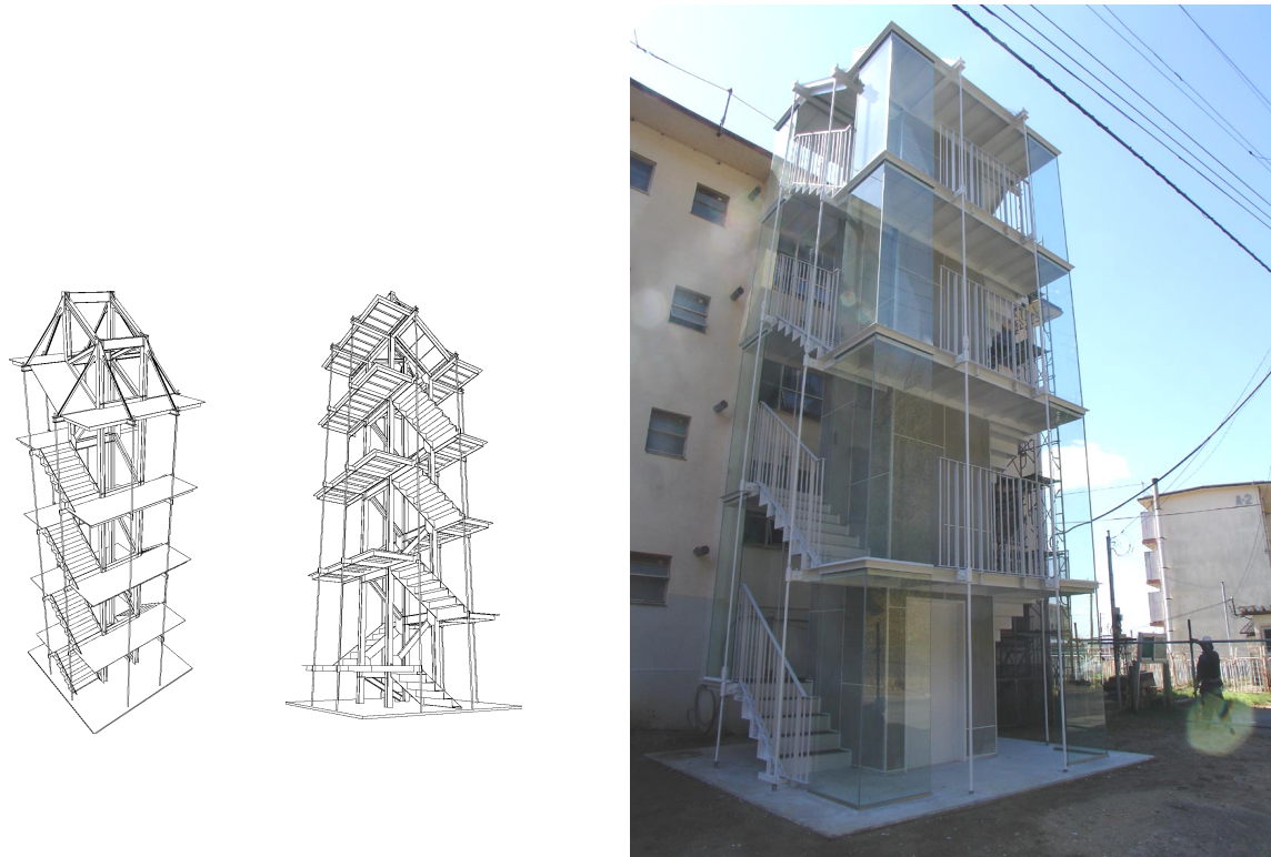
Figure 3. Structural diagrams of new system and photograph of the new elevator addition system applied
