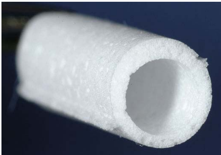
Figure 2.1: Example of a biodegradable vascular scaffold (biodegradable polyurethane foam, porosity > 95%, 0.5 cm diameter, 2.5 cm length).
