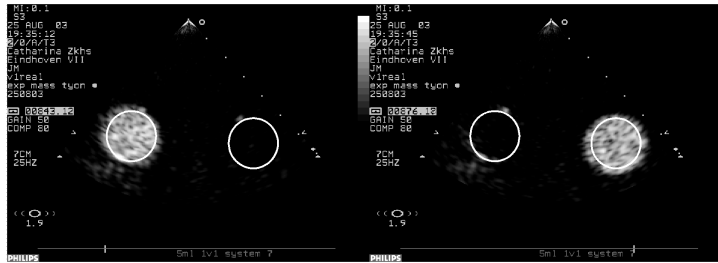
Figure 5.18: Two B-mode frames showing the passage of the contrast bolus through the first tube (left frame) and the second tube (right frame). A ROI is placed on each tube for the acoustic intensity measurement.
