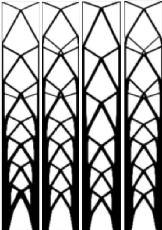
Fig. 15 Optimal topologies: left to right: SISO, MIMO (2-norm), MIMO (Nuclear norm), and MIMO (Frobenius norm)
