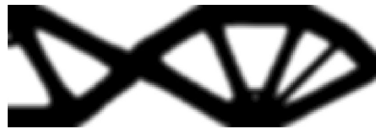
Fig. 9 SIMO formulation—Optimal topology: 2-norm, N -norm, and F -norm
