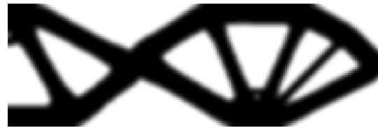
Fig. 7 MISO formulation—Optimal topology: 2-norm, N -norm, and F -norm
