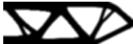
Fig. 12 Sigmund's 88-line code solution using the multiload case option
