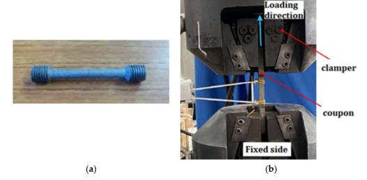
Figure 2. (a) A sample for uniaxial tensile tests; (b) testing setup.
