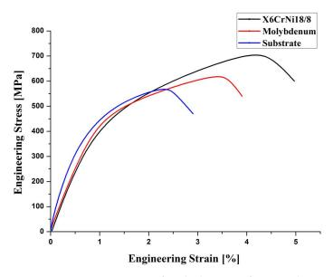
**Figure 6.** Stress–strain curves of studied coatings from tensile tests.
