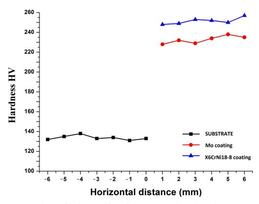
Figure 7. Hardness profiles determined for studied coatings using the Vickers scale.
