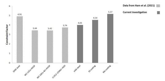
**Figure 8.** Chart with constraint factor values determined for current investigated arc-sprayed and HVOF coatings studied in reference [15].
