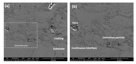
**Figure 5.** (a) Cross-sectional SEM image of the as-sprayed X6CrNi18-8 stainless steel coating; (b) zoomed area used to clarify the structural features.
