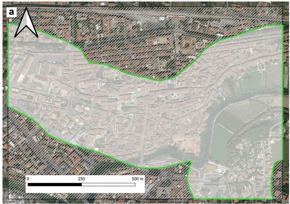
Fig. 9 Map (a) and 3D solid model (b) indicating zones with 1D and 2D seismic response schemes in the Rieti historical center (green and red colors, respectively, in transparency)
