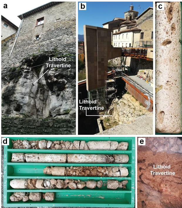
Fig. 2 Lithoid travertine (calcareous tufa, sensu Madonna et al., 2021) outcropping in Rieti: a, b travertine platform outcropping in the historic center; c, d piece of a core drilled in the center of Rieti, near the town hall; and e travertine outcrop at the base of an ancient building, in the historic city center
