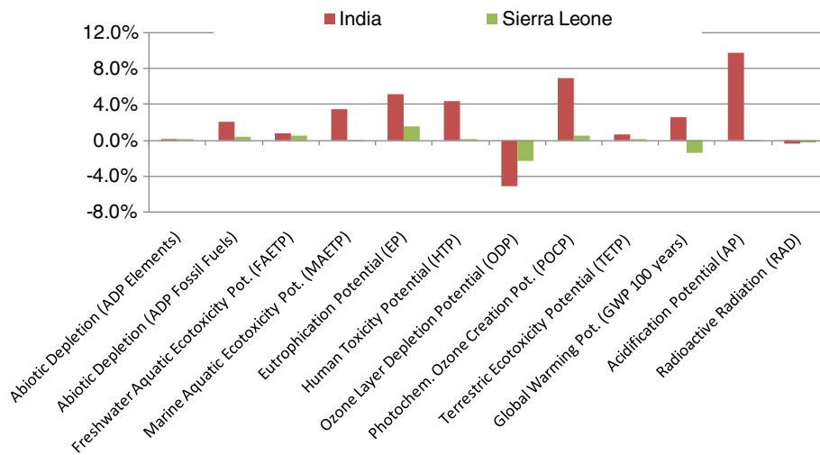
Figure 6 LCA results for different remanufacturing localizations - India and Sierra Leone relative to Germany (alternative 1, conventional-remanufacturing only).
