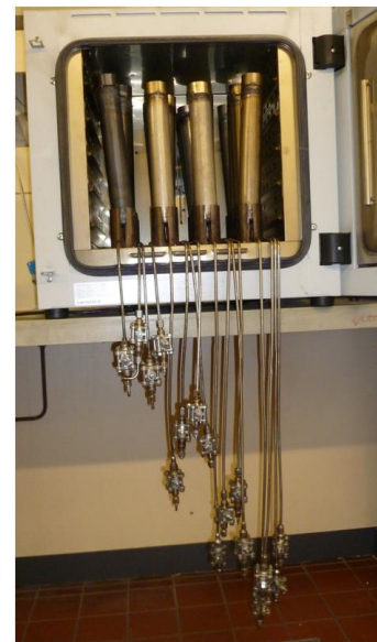
Figure 2: Photo of the autoclaves in the oven
