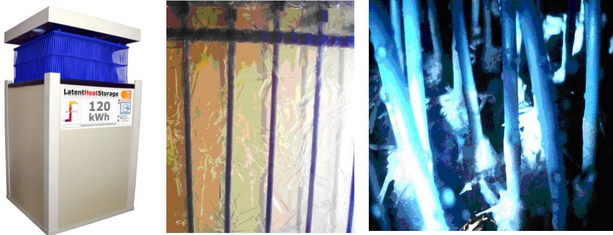
Figure 5: Latent heat storage and capillary matrix surrounded by crystallized salt hydrate
