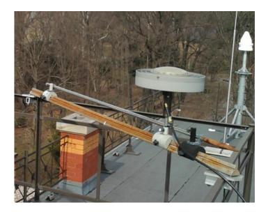
Figure 3.2: Equipment for the horizontal movement experiment of a GNSS antenna
