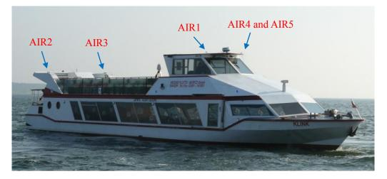
Figure 8.3: The ship used and the position of GNSS receiving equipments
