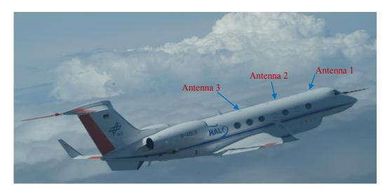
Figure 5.1: Multiple GNSS antennas mounted on the HALO aircraft (DLR, 2013a)
