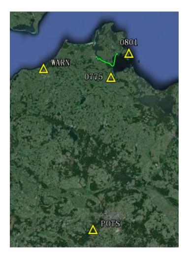
Figure 5.4: The track of the ship (green curve) and the positions of reference stations (yellow triangles) for the Baltic Sea shipborne gravimetric experiment on June 18. 2013
