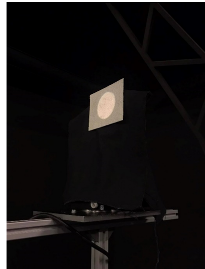
Fig. 2. Photograph of the sample and sample holder, showing the circular light spot with a diameter of 7.5 cm on the test sample at perpendicular incident.
