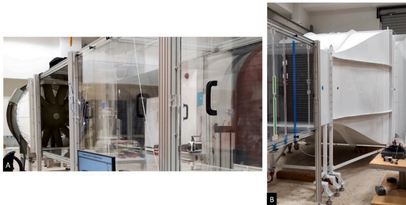
Fig. 7. RÜZGEM C3 wind tunnel: views towards a) the test section, and b) the settling chamber.
