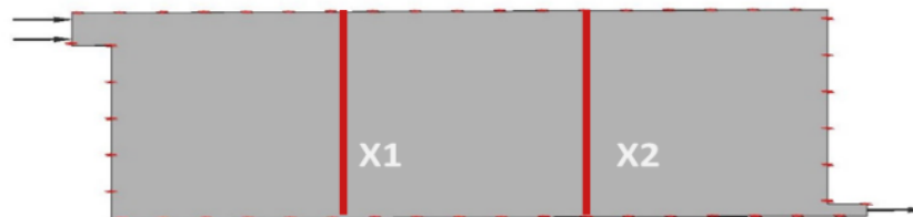
Figure 28: Schematic Cross-Section of the Demonstration Room Highlighting the Positions of Two Sensors, Indicated as X1 and X2
