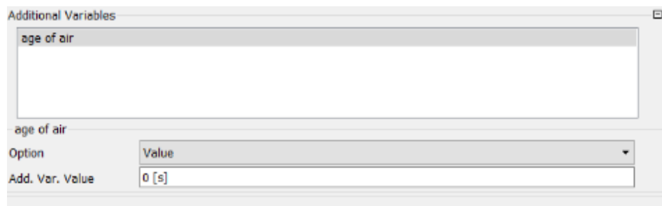
Figure 35: Step-by-step process for calculating 'Age of Air' within Ansys CFX using the CFX-Pre-module.
