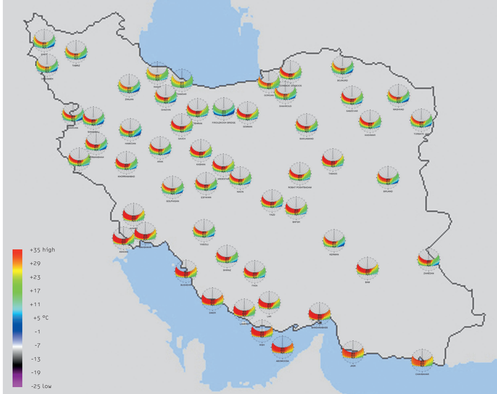
Fig. 56: Average hourly temperature in Iran (from 21 June to 21 December) based on long-term daily minimum and maximum temperature averages calculated by SOLARCHVISION
