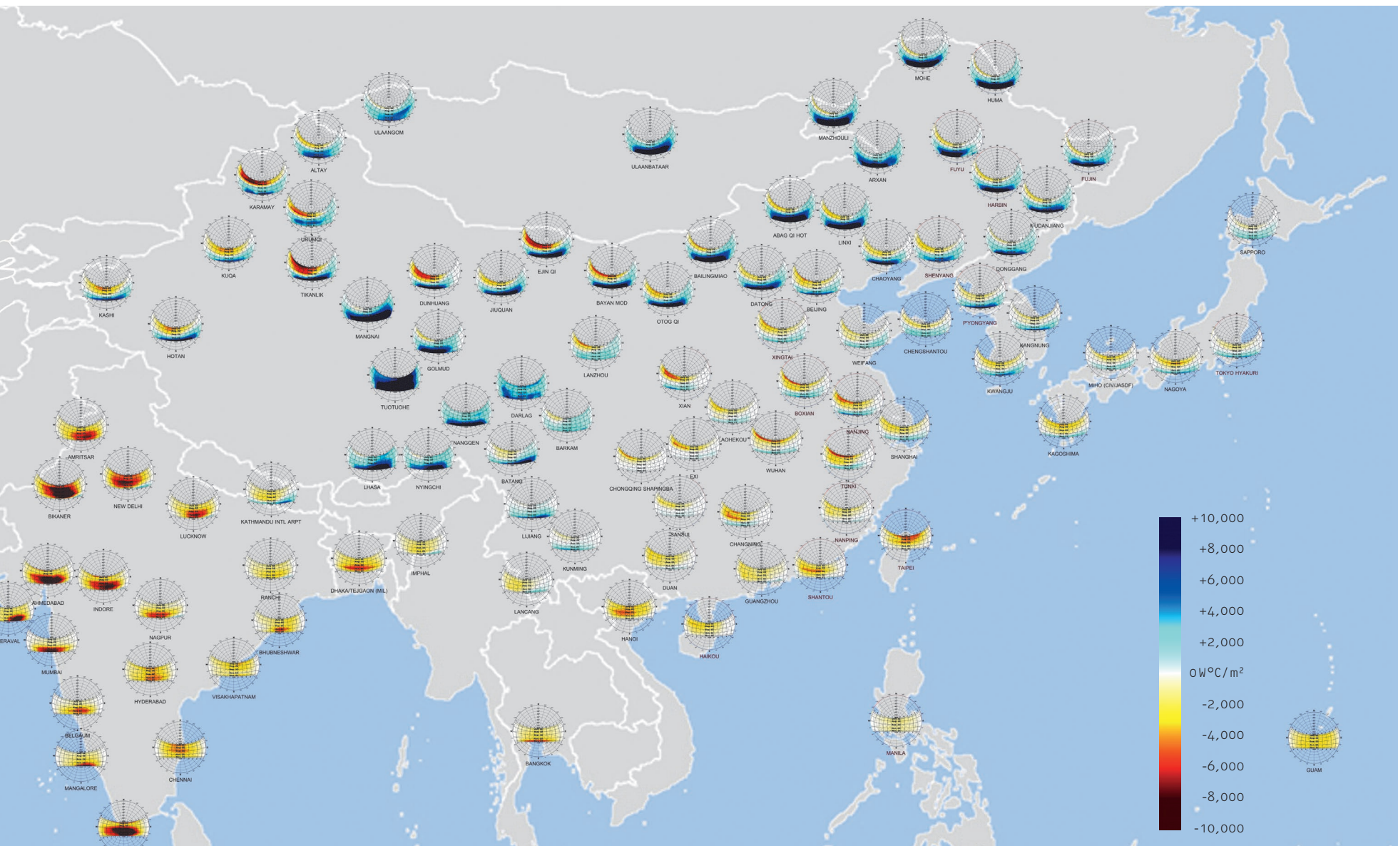
Fig. 83: Average hourly positive and negative effects of direct solar radiation from June 21 to December 21 in East Asia (China, India, Japan, etc.)
