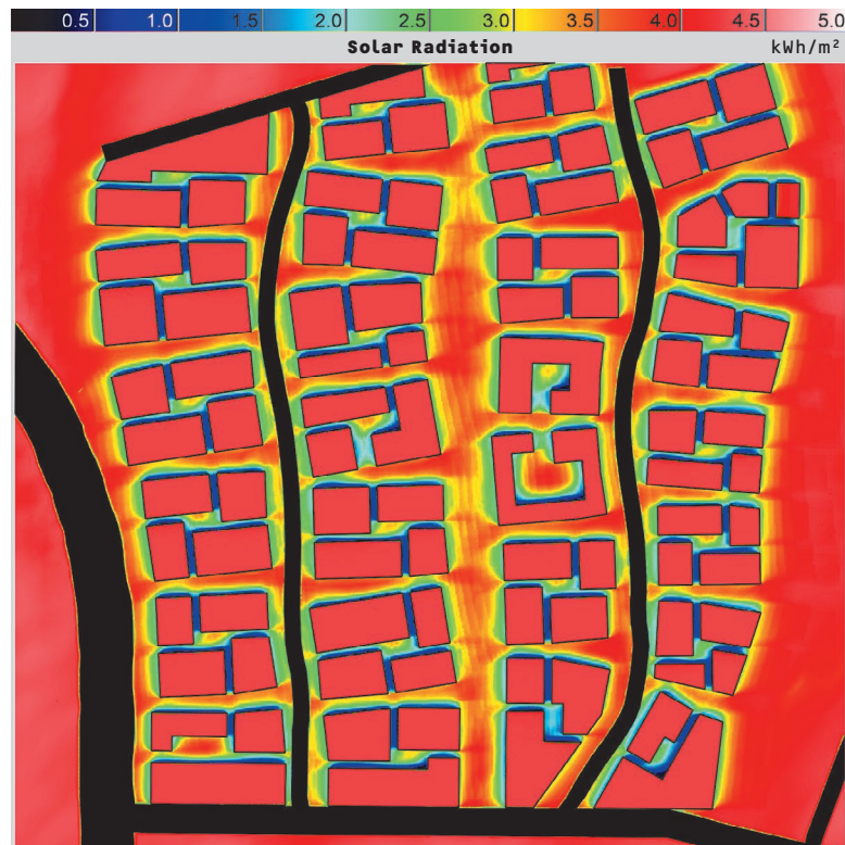
Fig. 299: SOLARCHVISION active analysis, annual solar radiation model of the Shahre Javan Community
