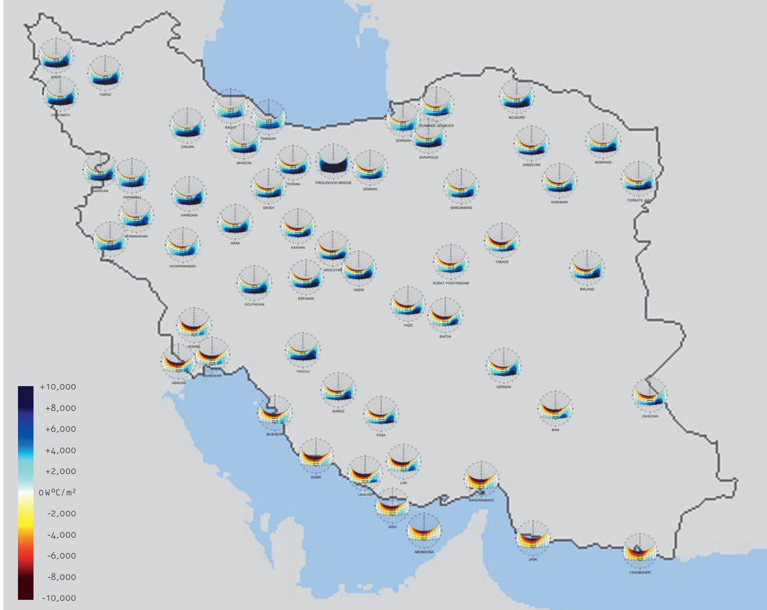
Fig. 86: Average hourly positive and negative effects of direct solar radiation from December 21 to June 21 in Iran
