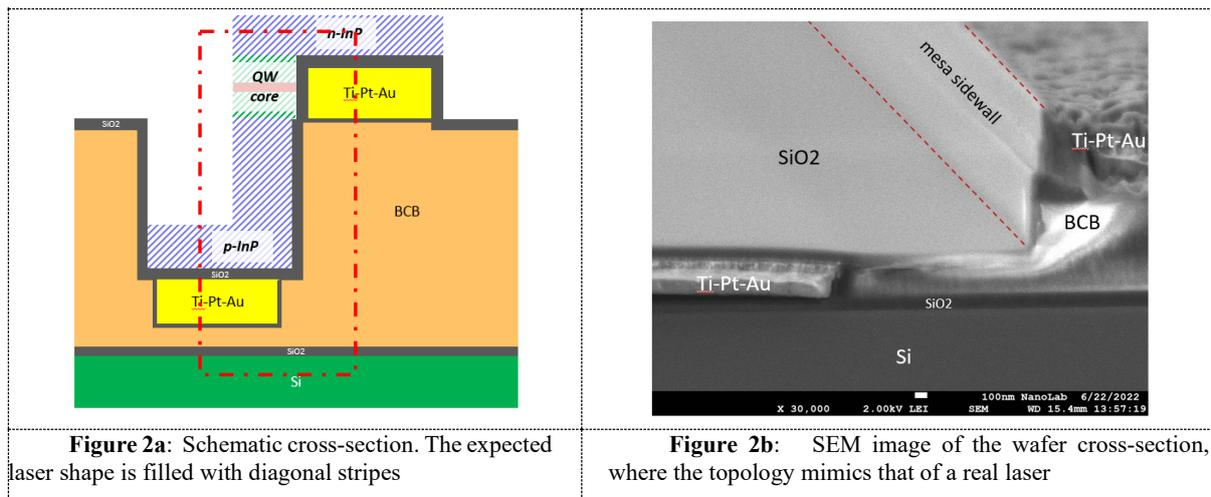
**Figure 2a:** Schematic cross-section. The expected laser shape is filled with diagonal stripes
