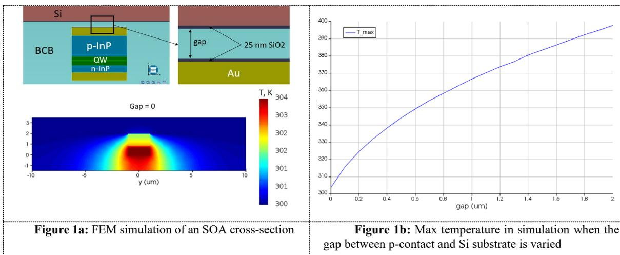
Figure 1a: FEM simulation of an SOA cross-section
