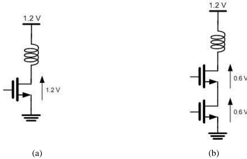
Fig. 98 The maximum voltage swing a) C.S. b) Cascode.
