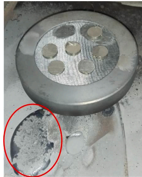
Fig. 4. Second attempt at Sn wetting of the W meshes due to spilling of Sn (red circle) during the first wetting.
