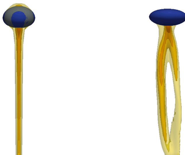
Fig. 2. Visualizations of the concentration profile for a spherical bubble (Eötvös number of 1, Morton number of 10^{-3} and Peclet number of 10^6 ) and a wobbling bubble (Eötvös number of 10, Morton number of 10^{-11} and Peclet number of 9 \cdot 10^5 ) on the left and right, respectively. The concentration value increases from yellow to orange and the blue contour is the bubble.
