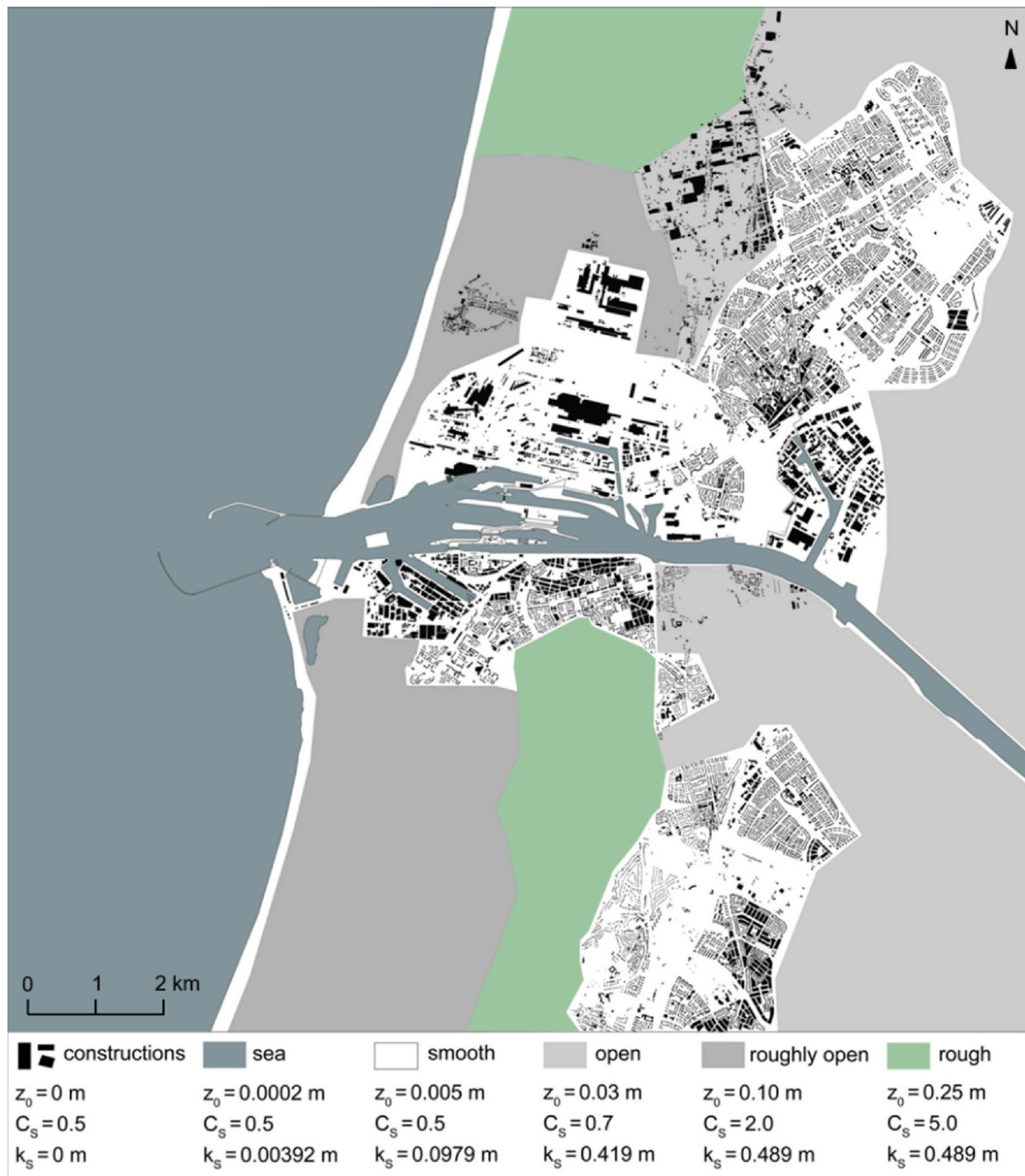
Fig. 7. Aerodynamic roughness length ( z_0 ), roughness constant ( C_s ) and equivalent sand-grain roughness height ( k_s ) for patches with different terrain roughness categories.
