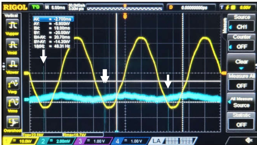
Figure 13-9 Oscilloscope plot of LV to MV electrical discharges
