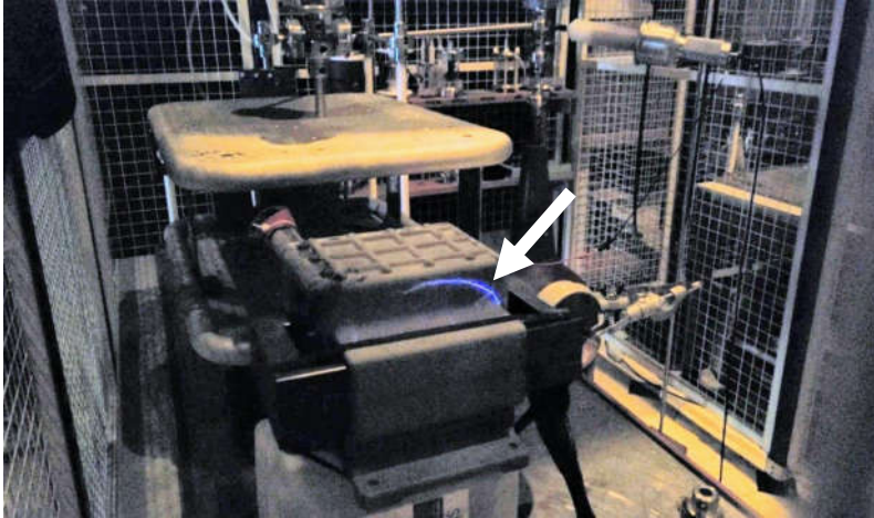
Figure 13-12 Surface discharges on DAB transformer during 60 kV PEAK AC test
