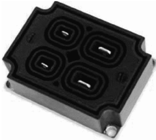
Figure 9-3 Wide bandgap device packaging [23]
