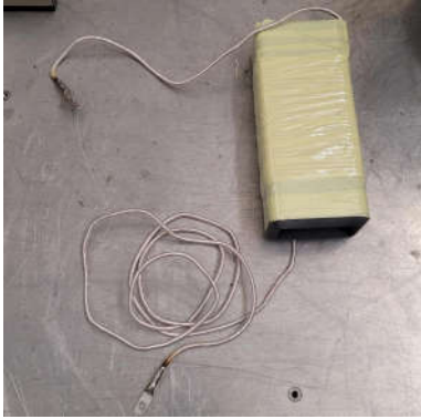
a. LV winding insulated with tape
