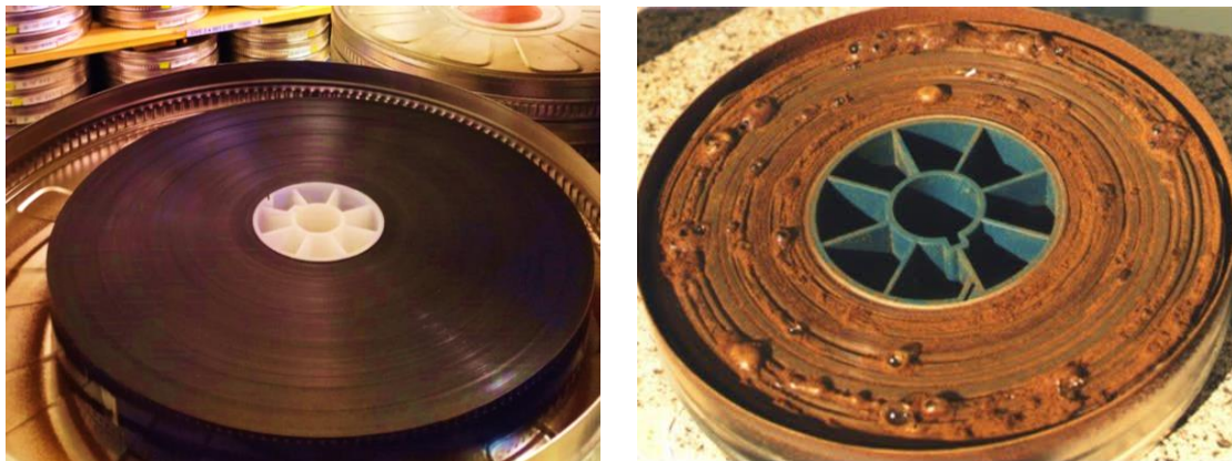
Figure 1. Left: healthy nitrate film [picture taken by author]; right: highly decomposed nitrate film [3]
