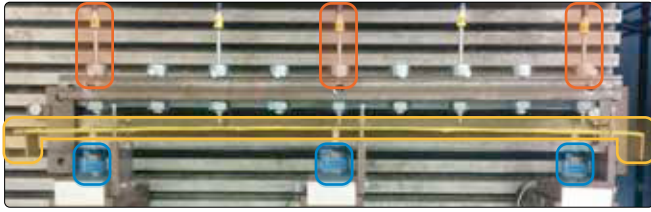
Fig. 2. Prototype experimental setup. The moving part, i.e., the flexible beam, is equipped with yellow tape and is outlined with (■). The beam is actuated by three voice coil actuators (●), and five fiber-optic displacement sensors, of which three are used (■). The steel beam is held up by four wire flexures from the table upwards, and one sideways on the left.
