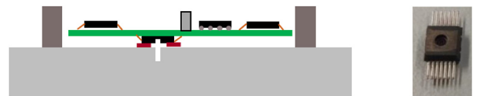
Fig. 36. Basic concept (left) of a sensor (right) to monitor the pressure inside a battery cell.
