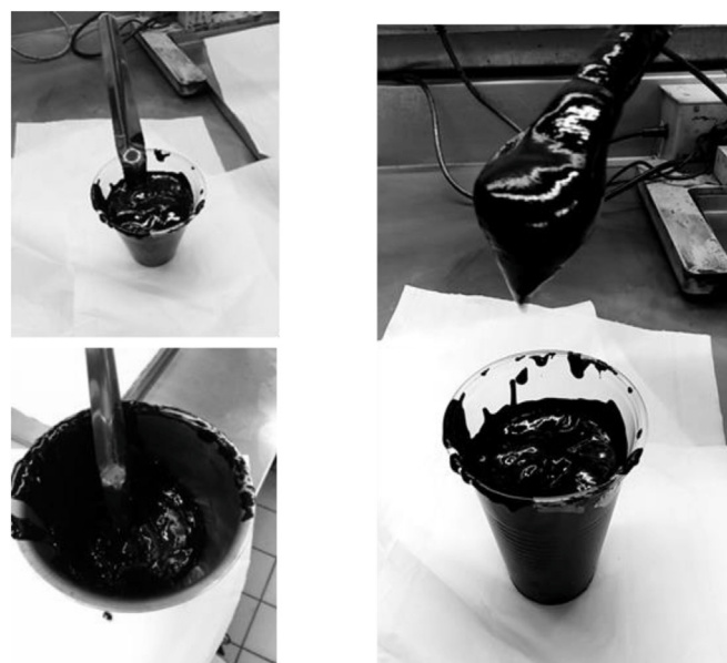
Fig. 31. Lab scale preparation of electrode ink.
