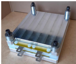
Fig. 3. Cell Holder to mimic module environment.
