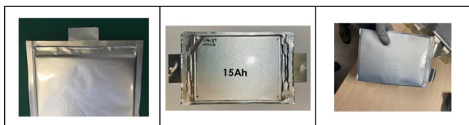
Fig. 32. 3 generations of cells for DEMOBASE project with opposite (LS, LU and MU types) tabs and “rabbit type” tabs configuration (Mter type).
