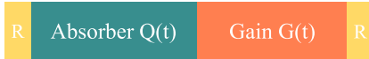
Fig. 1. Schematic overview of a laser with saturable absorber and gain section laser. The absorber and gain elements are surrounded by mirrors R to create an optical cavity.
