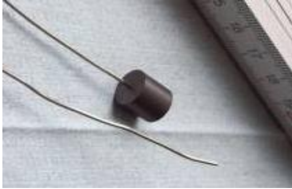
Figure 8: Picture of the graphite bolometer used in the MISTRAL to measure the microwave power [12] . The height and the diameter are both 10 mm.
