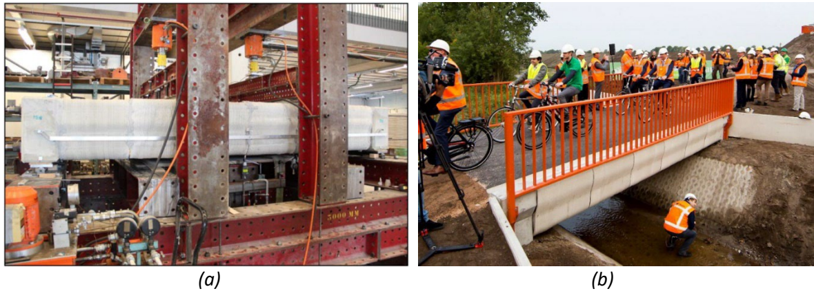
Figure 1-1: The scale model in 4-point bending test set-up(a) and the completed bridge at the opening of Gemert 3DCP bridge(b), as described in [11].
