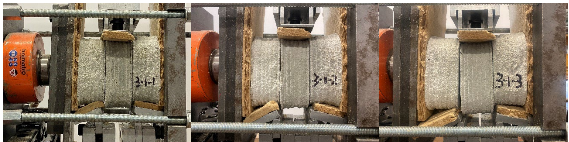
Figure 7-6: The shear test for straight connection without interlayer material.
