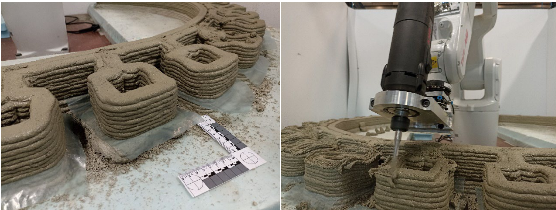
Figure 3-4: The printing process(left) and milling process(right) of printed bricks.
