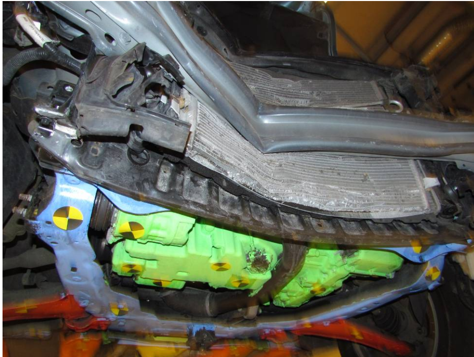
Figure 3.13: Deformation of bumper beam in modified SUV.
