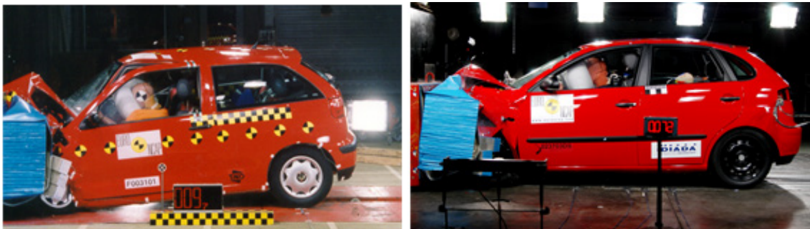
Figure 2.2: Left: Model year 2000 Seat Ibiza which suffers from severe compartment deformation noticeable by the A-pillar collapse and the front wheel displacement. Right: Model year 2003 Seat Ibiza with minimal compartment deformation [Euro NCAP 2013].
