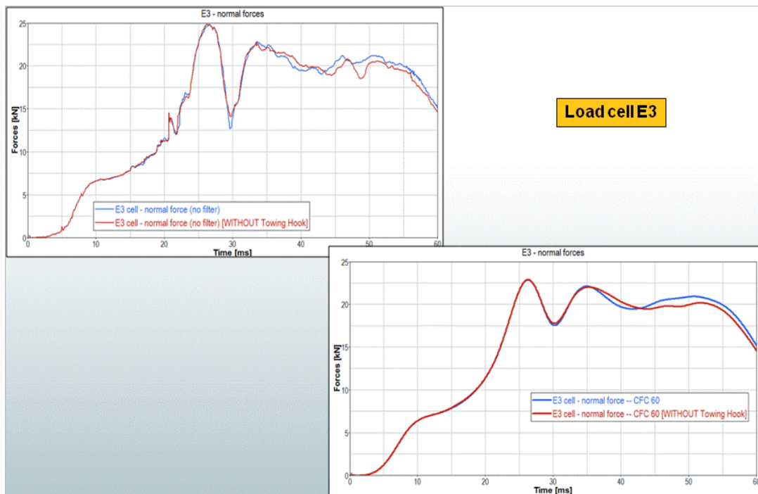
Figure 4.12: Load on (lower) directly impacted cell: comparison between runs with and without towing hook mounting.
