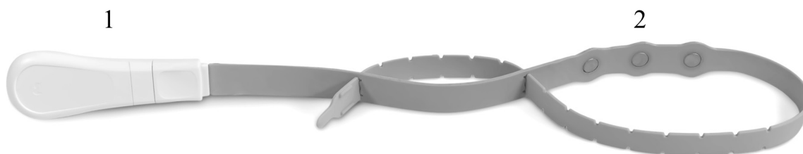
Figure 2 The Bambi® belt is a wireless non-adhesive belt designed for cardiorespiratory monitoring of (pre)term infants. The three dry electrodes 2 measure electrical activity of the diaphragm via transcutaneous electromyography. These data are wirelessly transmitted with the sensor module 1 to a receiver module that processes the diaphragm activity to obtain the electrocardiogram, respiration signal, heart rate and respiratory rate.
