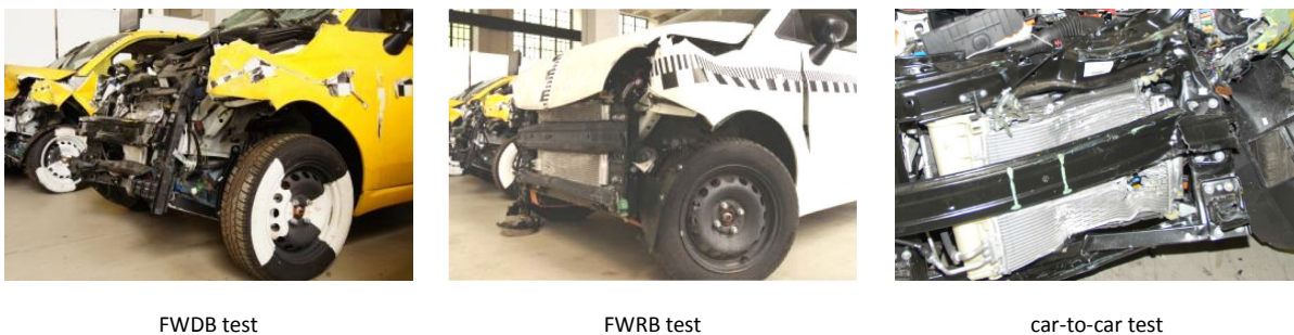
Figure 2.6: Comparison of front structure deformation pattern in different frontal impact tests.
