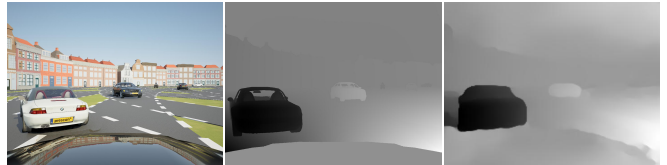
Fig. 2: Simulated camera input (left), ground truth (center) and CNN estimated (right) horizontal optical flow.
