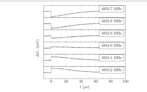
**Figure 2.** The change in the cavity reflection voltage  $\Delta V_r \equiv V_r - V_0$  as a function of time *t* for six different applied frequencies  $\omega/2\pi$  to the cavity, due to the creation of a UCP at t = 0, with  $V_0$  being the average reflection voltage for t < 0.
