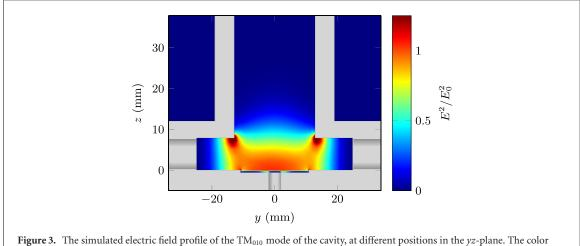
Figure 3. The simulated electric field profile of the  $TM_{010}$  mode of the cavity, at different positions in the *yz*-plane. The color indicates the square of the normalized electric field amplitude  $E/E_0$ , with  $E_0$  being the field amplitude at position x = 0 mm, y = 0 mm, and z = 2 mm. Reproduced from [17]. CC BY 4.0.
