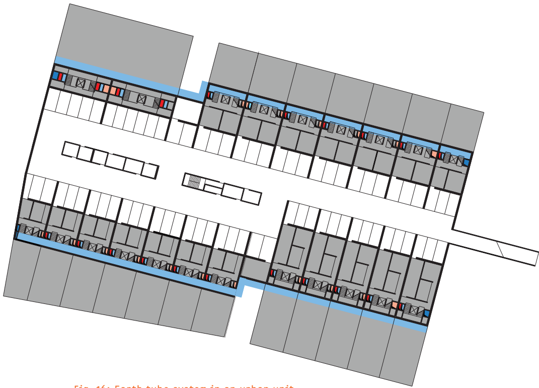
Fig. 16: Earth tube system in an urban unit
