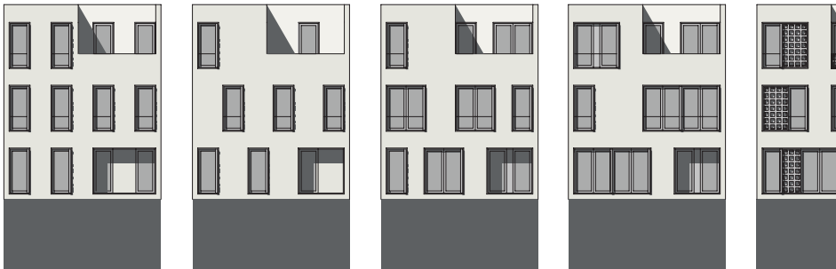
Fig. 18: Study of different south façades for 7.5 m building type
