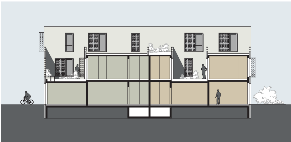
Fig. 12: Section through a 9m-type building with two dwelling units, each with its own private courtyard
