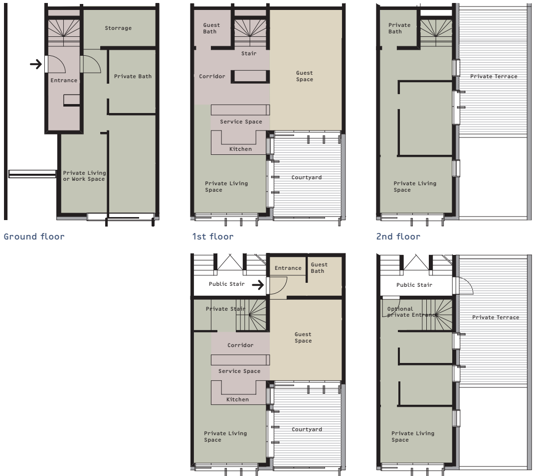
Fig. 13: Floor plans of a two and three-storey dwelling in a 9m-type with a private courtyard and zoning inside the dwelling
