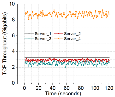
Fig. 7. Real-time TCP traffic monitored at servers for 120 seconds.
