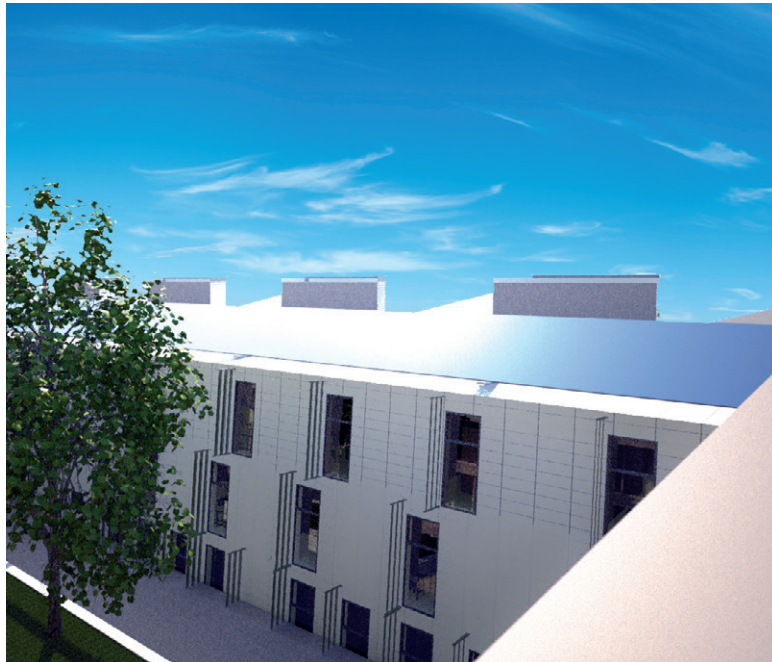
Fig. 67: Fixed shading devices for different cardinal directions Fig. 68: Fixed shading devices on north façade
