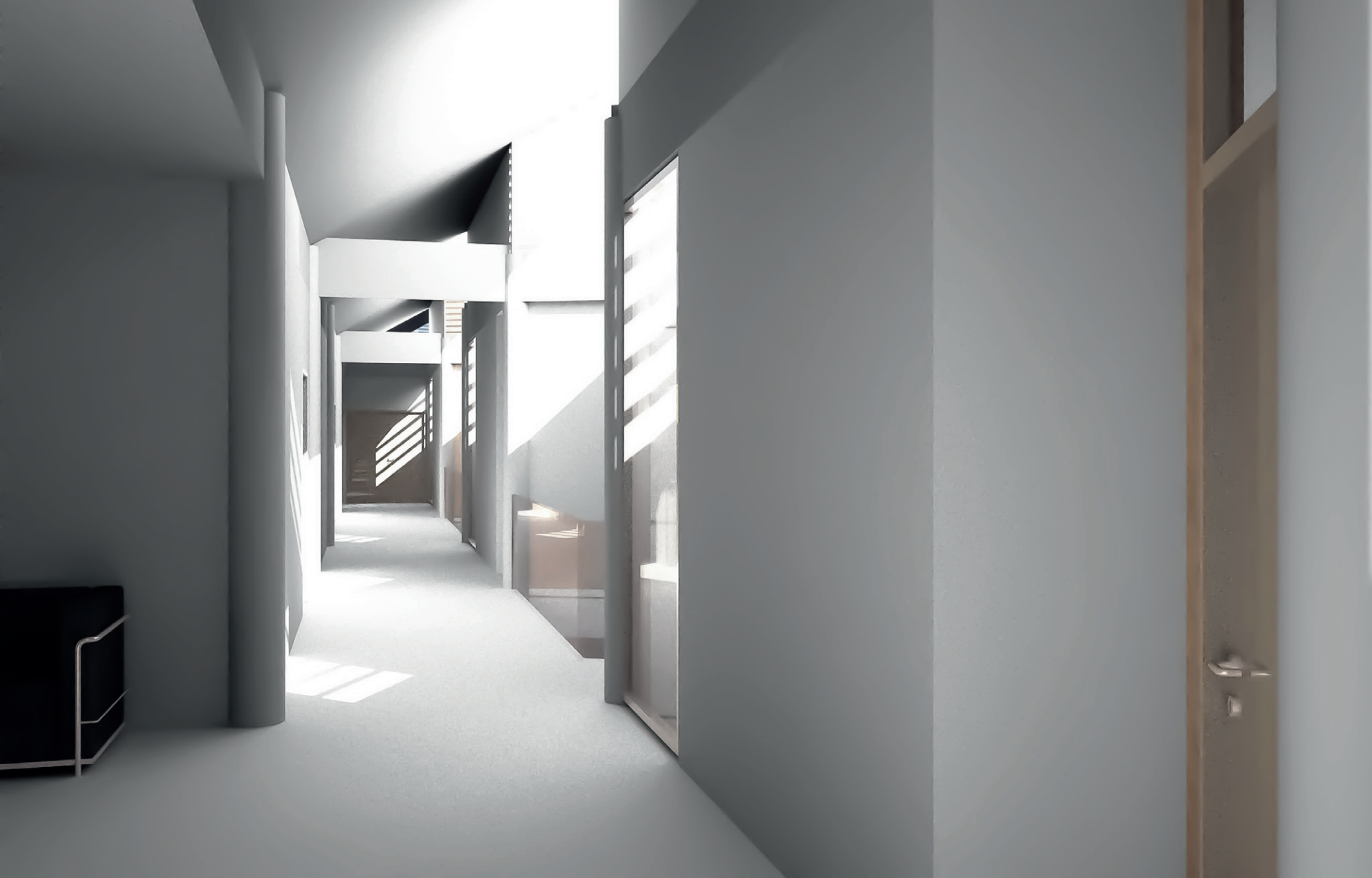
Fig. 120: Daylight provision through skylights
