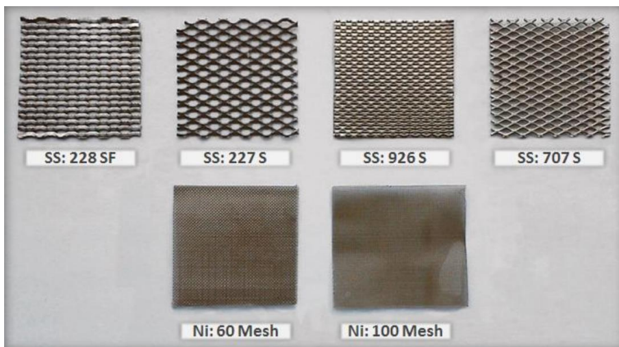
Figure 1: mesh electrodes used in this work. The top row consists of 316 stainless steel expanded meshes, the bottom row of nickel wire meshes. The ratio A_{mesh}/A_{plate} , as well as the geometric parameters are given in table 4a and table 4b.
