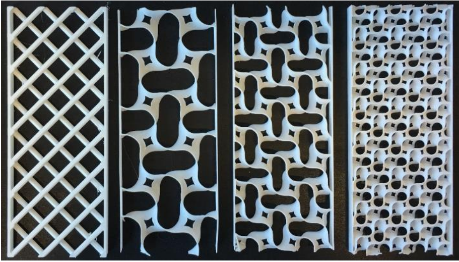
Figure 5: 3D printed turbulence promoters used in this work. From left to right: Tube grid promoter, large gyroid, medium gyroid and small gyroid. These are the 100 mm long variants, 250 mm long variants were also used.
