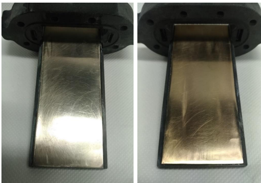
Figure A6: Yellowing of the electrodes in the printed cell. Left: before the 17h reduction experiment shown in figure 7, right: after 17 hours of hexacyanoferrate(III) reduction in 0.5M KOH.
