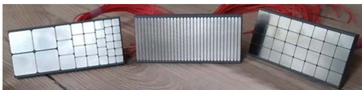
Figure 1: Segmentation patterns of electrode. left: focused, middle: series, right: matrix. The electrodes are installed in such a way that the flow crosses the electrodes from the right to the left.
