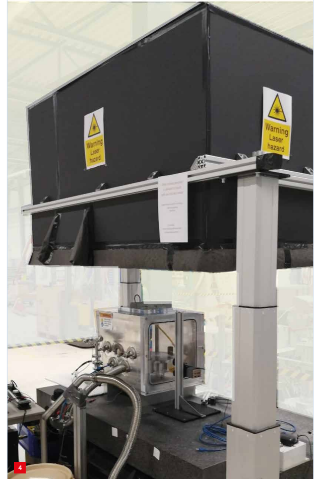
Experimental set-up to study the particle-gas interaction with the possibility to control pressure, temperature and temperature gradient. The photo shows all the main components of the set-up: the vacuum chamber (in the middle) on top of an optical table, and a special cover (black box above the chamber) closing the chamber during the experiment for safety and optical background reduction [5].
