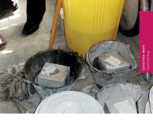
Test cubes for pressure strength test improperly stored No proper equipment for a concrete laboratory
