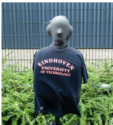
Fig. 2. B&K HATS with windshields.
