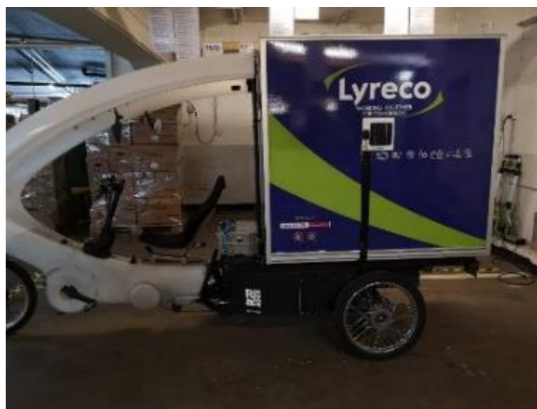
Fig. 3.3-8 The «Rikscha Taxi» with a cargo box showing the left irradiance sensor.
