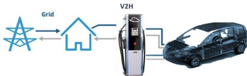
Fig. 4.3-15 Principle scheme for V2H service [illustration based on [6]]
