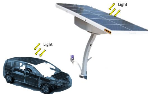
Fig. 4.3-13 PV canopy infrastructure enhanced for PV-powered vehicle
