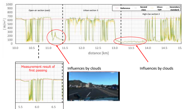
Fig. 3.2-1 September 20, 2018 (Day 1) in Sapporo: Measurement results for solar irradiance during the First run [1]
