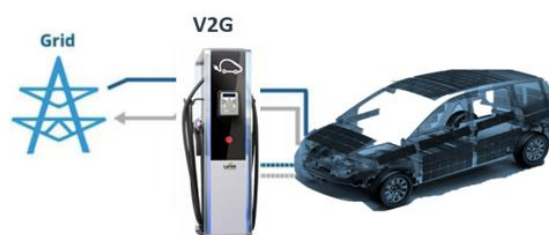
Fig. 4.3-14 Principle scheme for V2G service [illustration based on [6]]
