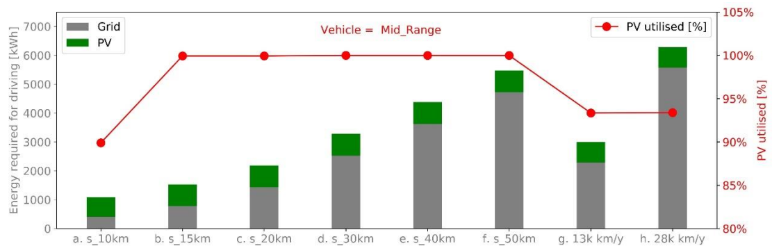
Fig. 2.2-21 The total kWh utilised for driving divided into Grid and PV charging (left axis) and the percentage of generated PV energy that has been utilised (right axis) for Amsterdam and the mid-range vehicle
